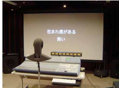
Figure 13 The recording setup using a dummy head microphone in the same environment
