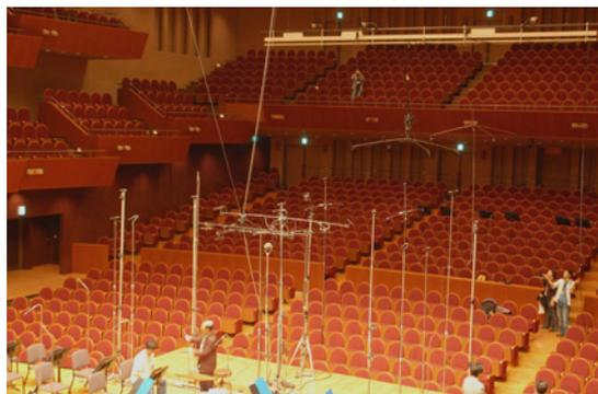
Photo4-1 Placements of the Microphone-Arrays
